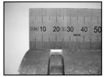
Measure the gasket seat length A and the groove width B using a ruler, a scale or a tape with linear scale to ensure the dimensions are within the tolerances specified in column 3 and column 4 of table 2.
