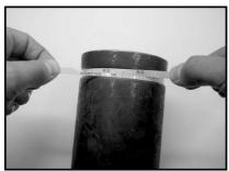
Measure the groove bottom using a diameter tape, a circumference tape or a vernier caliper measuring at 0° and at 90° on the circumference to ensure that the groove bottom diameter C or the groove bottom circumference is within the tolerances specified in column 5 of table 1.
