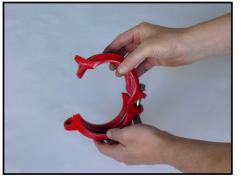
Bolts and nuts should now be removed from one side of the coupling, if not already done, and the bolts and nuts on the other side should be loosened, until the thread of the bolt no longer protrudes over the nut.
