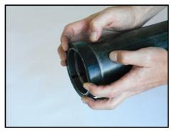
Push or pull the gasket carefully over the pipe end until the cut edge of the pipe end is visible again.
