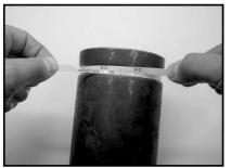
Measure the groove bottom using a diameter tape, a circumference tape or a vernier caliper measuring at 0° and at 90° on the circumference to ensure that the groove bottom diameter C or the groove bottom circumference is within the tolerances specified in column 5 of table 2.
