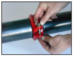
Insert the remaining bolt into the bolt holes and tighten the nut by hand.
