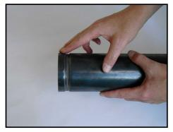
The pipe ends must be burr-free to avoid damage to the gasket during assembly.
