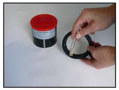
To avoid gasket pinching, the outside of the gasket and the inside of the coupling half-shells as well as the inside of the sealing lips and the outside of the pipe ends must be lightly lubricated.
