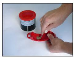
Cover the inside of both half-shells of the coupling with a thin layer of lubricant.
