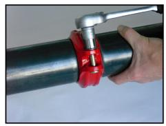
Tighten the coupling nuts evenly and by alternating sides, until the angle-design bolt pads meet metal to metal. To achieve optimum sealing performance and stability, the nuts must be tightened with the specified torque corresponding to
